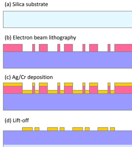
Fig.2. Fabrication process.
