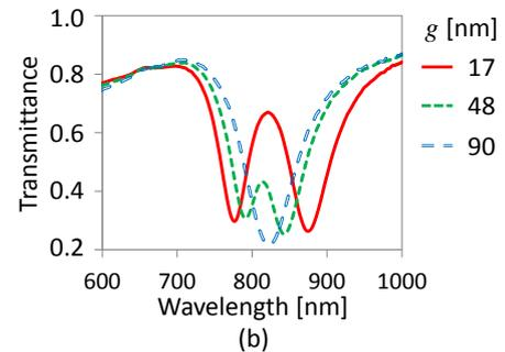
Fig.3. (a) SEM image of the fabricated EIT metamaterial. (b) Measured transmittance spectra.
