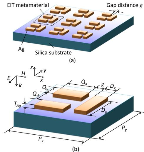
Fig.1. A schematics of (a) a planar EIT metamaterial array and (b) a unit of the EIT metamaterial structure with the geometrical parameters:  $D_x = 100 \text{ nm}$ ,  $D_y = 195 \text{ nm}$ ,  $Q_x = 170 \text{ nm}$ ,  $Q_y = 80 \text{ nm}$ ,  $Q_d = 80 \text{ nm}$ , and  $T_{Ag} = 45 \text{ nm}$ . The periods in both the  $x$  and  $y$  directions,  $P_x$  and  $P_y$ , are 470 nm.
